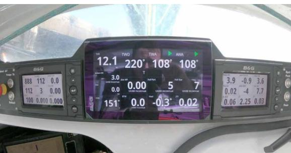
**Data is a critical driver in IMOCA performance and safety. Load sensing on all sail tack points and fibre optic sensing in the foils allows the skipper to stay within the limits.**
